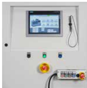
Siemens S7 controls
