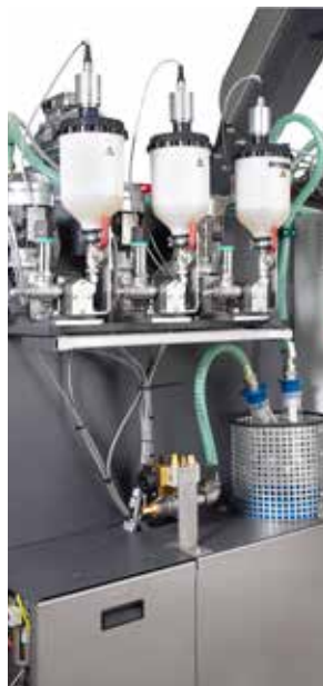
Colour and additive dosing
