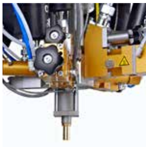
Mixing head, pressure regulation valve
