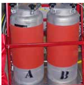
Electrical heating mats
