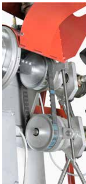
Pump drive with cog wheels
