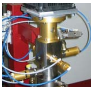
Mixing head with water cooling
