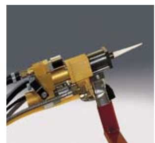
Mixing head with dynamic mixing
